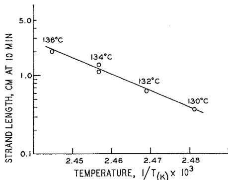
Figure 4 Growth rate of transparent polyethylene strands, capillary I.
