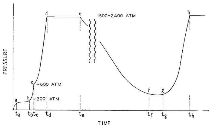
Figure 1 Instron rheometer pressure trace.
