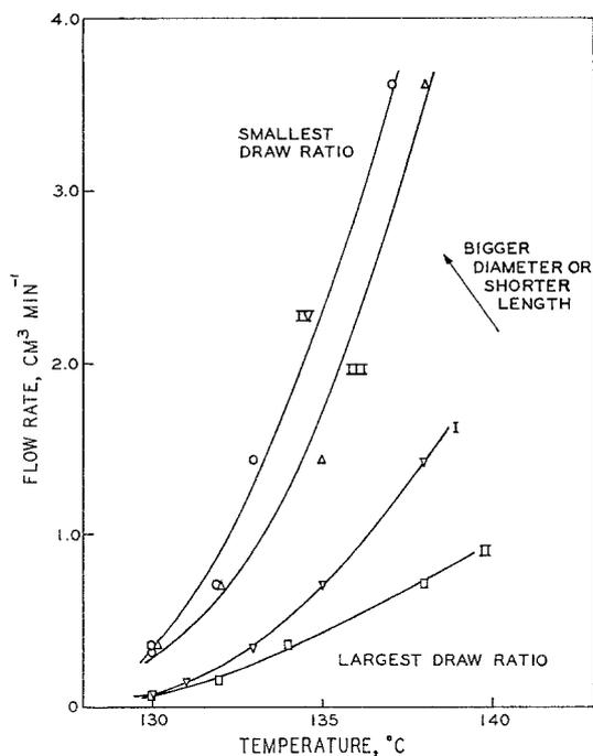
Figure 5 Combination of volume flow rate and temperature needed for reservoir crystallization for different capillary geometries, I, II, III and IV.
