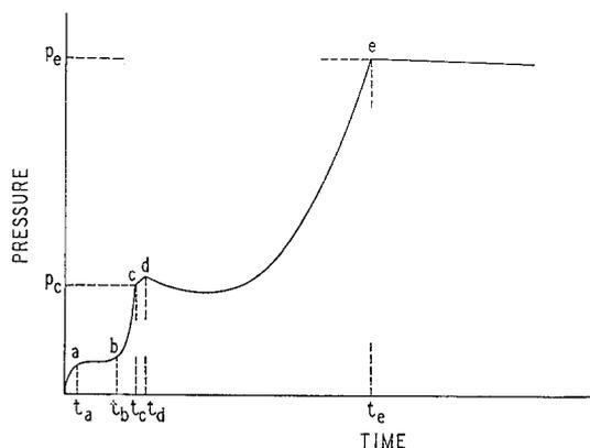
Figure 2 Instron rheometer pressure trace, combination method.
