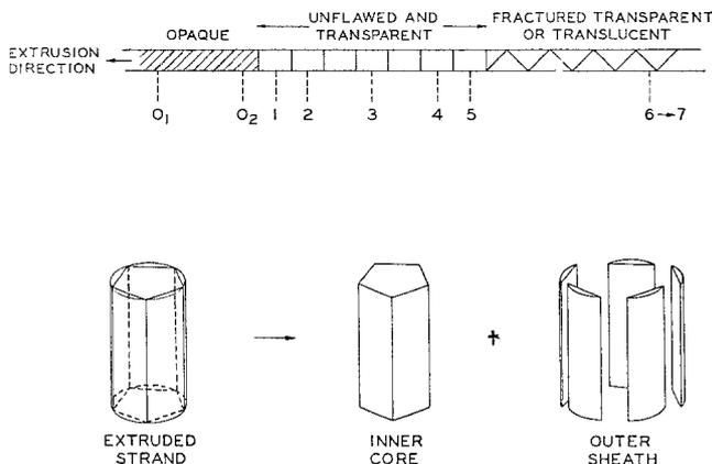
Figure 7 Sections of special polyethylene morphology.
